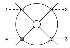
Possible movements. w motor pairs 1, Adjacent motor pairs: 1&2, 2&3, 3&4, 4&1 can be moved synchronously in the same direction.
